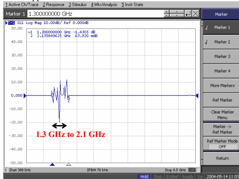
Figure 1. Trace shows noise around 1.3 GHz to 2.1 GHz at preset setting.
